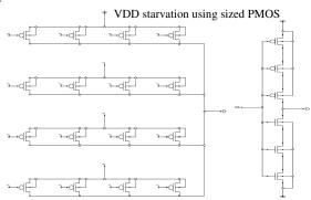
Figure 6: Custom-Cell Optimized PUF ("CO")
