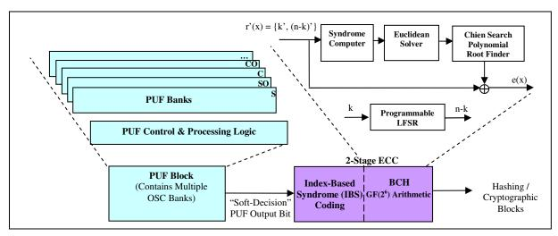
Figure 2: PUF Cryptographic Key Generation ASIC Block Diagram
