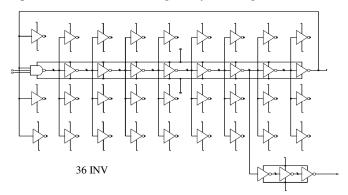
Figure 3: Standard-Cell PUF ("S")
